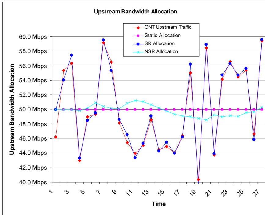
When implementing SR-based allocation, the OLT can measure the incoming traffic from the ONT and has full visibility into the upstream queue occupancy of the ONT. The SR-based allocation tracks ONT needs well and empties the ONT upstream queue in a timely manner. As seen in Figure 8 and Figure 9, the upstream latency is kept low and relatively constant, and there is no risk of queue overflow and packet loss.
