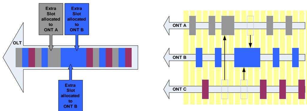
A good DBA algorithm quickly adjusts the upstream bandwidth allocation to the ever-changing traffic scenarios. At any given time slot, sufficient bandwidth would be allocated to certain ONTs (or certain services). In other time slots, the bandwidth would be allocated to other ONTs or other services, maximizing utilization of the PON bandwidth.
