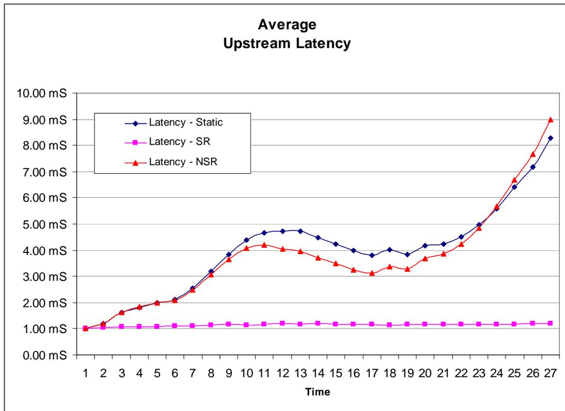
**Figure 9 Average Upstream Latency with SR DBA**
